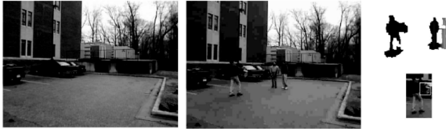
Fig. 1.1 Background subtraction identifies groups of pixels that differ significantly from a background model. The method is most useful for some some cases of surveillance, where one is guaranteed a fixed viewpoint and a static background changing slowly in appearance. On the left, a background model; in the center, a frame; and on the right, the resulting image blobs. The figure is taken from Haritaoglu et al. [146]; in this paper, authors use an elaborate method involving a combination of thresholds to obtain good blobs. Figure 1.2 illustrates a method due to these authors that obtains a kinematic configuration estimate by parsing the blob. Figure from “W4: Real-time surveillance of people and their activities”, Haritaoglu et al., IEEE Trans. Pattern Analysis and Machine Intelligence, 2000, © 2000 IEEE.
