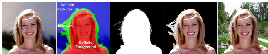
Fig. 1.1 A matting example. From left to right: input image; user specified trimap; extracted matte; estimated foreground colors; a new composite. Results are generated by the Robust Matting algorithm [49].
