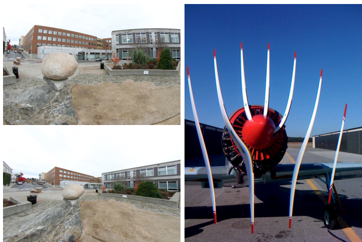
Figure 1.4: Common deviations from pinhole camera model. Left: a fish eye lens exhibiting large radial distortion (top) and a rectified version of the same image after removing radial distortion (bottom). Right: rolling shutter artifacts caused by a fast moving object in the scene [155].
