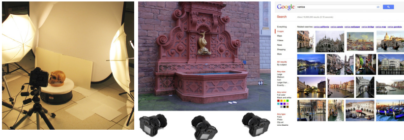
Figure 1.3: Different MVS capture setups. From left to right: a controlled MVS capture using diffuse lights and a turn table, outdoor capture of small-scale scenes, and crowd-sourcing from online photo-sharing websites.
