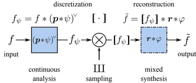
**Figure 1.3:** The main idea in generalized sampling is to broaden the analysis and reconstruction kernels by expressing these as mixed convolutions ( $\mathbf{p} * \psi$  and  $\mathbf{r} * \varphi$ ) with a pair of digital filters ( $\mathbf{p}$  and  $\mathbf{r}$ ) while retaining compact support for the functions  $\psi$  and  $\varphi$ .
