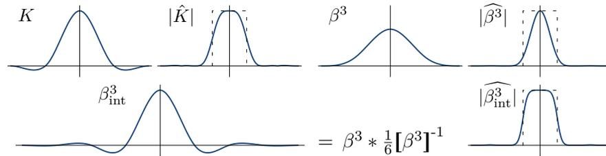
**Figure 1.4:** The traditional Keys cubic (Catmull-Rom spline)  $K$  has support 4 and a reasonably sharp frequency response  $|\hat{K}|$ . The cardinal cubic B-Spline  $\beta^3_{\text{int}}$  is a generalized kernel formed from the basic cubic B-spline  $\beta^3$  and a digital filter. The digital filter acts to widen support to infinity (though with exponential decay) and to significantly sharpen the frequency response.
