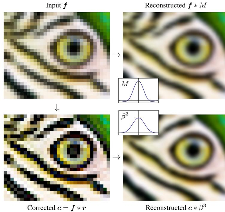
**Figure 1.6:** Reconstruction example. The top row shows the result of the traditional cubic Mitchell-Netravali filter  $M$ . The bottom row uses the generalized sampling approach, first applying a digital filter  $r = \left[\frac{1}{6}, \frac{4}{6}, \frac{1}{6}\right]^{-1}$  as a preprocess, and then reconstructing with the cubic B-spline  $\beta^3$  — which is less expensive to evaluate on a GPU than filter  $M$ .
