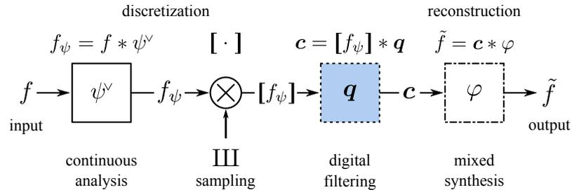
**Figure 1.5:** Generalized sampling adds a digital filtering stage to the pipeline. The output  $[f_\psi]$  of the sampling stage is convolved with a digital transformation filter  $q = p^v * r$ . It is the result  $c$  of this stage (and not  $[f_\psi]$ ) that is convolved with the reconstruction kernel  $\varphi$  to produce the output signal.
