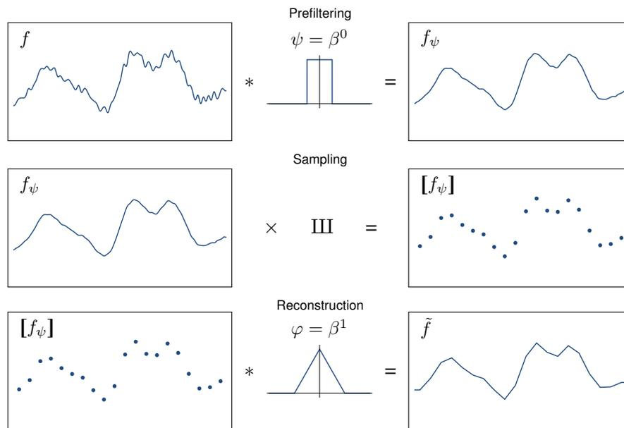
**Figure 1.2:** A continuous function  $f$  is prefiltered with analysis kernel  $\psi$  (here the box function  $\beta^0$ , not to scale). The resulting signal  $f_\psi$  is sampled into a discrete sequence  $[f_\psi]$ . The final output  $\tilde{f}$  is obtained by mixed convolution between the discrete sequence  $[f_\psi]$  and the reconstruction kernel  $\varphi$  (here the hat function  $\beta^1$ , not to scale).
