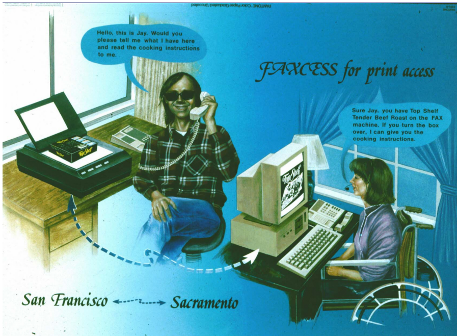
Figure 1.1: A diagram of the Faxcess system from the early 1990s for helping blind people interpret visual information. In this example, a blind person has taken a picture of the box for a frozen dinner with a digital scanner, and sent it to a human supporter who is reading the information to him over the phone. It is interesting to note that the supporter herself has a physical disability. While this was not called human computation or crowdsourcing at the time, it presaged many of these ideas.
