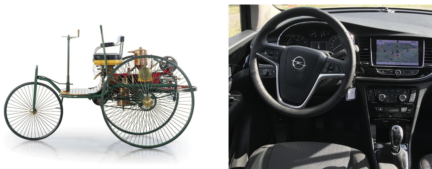
Figure 1.1: Human-machine interaction for vehicles has become more complicated over the years. On the left is the Benz's 1886 Patent Motorwagen, the world's first automobile (image by DaimlerChrysler AG, CC-BY-SA-3.0, via Wikimedia Commons). On the right is the interior of a 2017 Opel. The operator of the Benz interacted with the vehicle through inputs to control lateral and longitudinal position. The 2017 vehicle has myriad displays and inputs.
