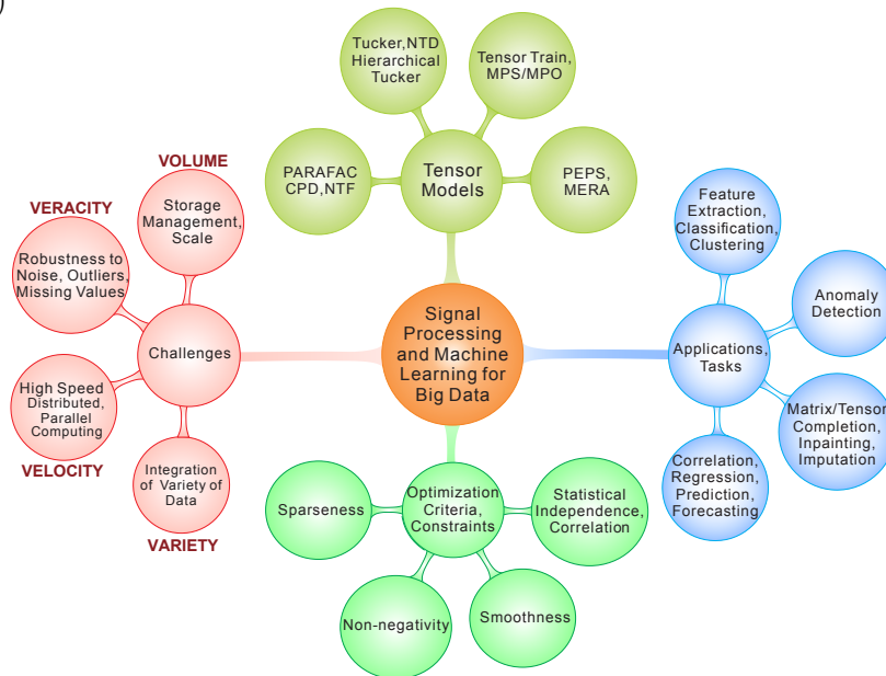
Figure 1.1: A framework for extremely large-scale data analysis. (a) The 4V challenges for big data. (b) A unified framework for the 4V challenges and the potential applications based on tensor decomposition approaches.
