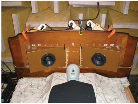
Fig. 10. Experimental setup for the snore ANC inside an acoustic chamber.
