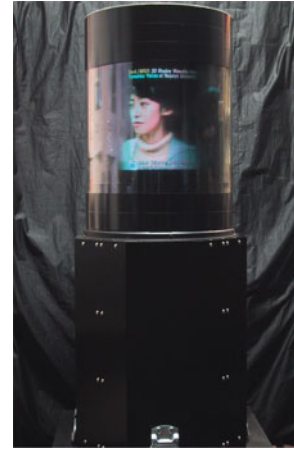
Fig. 30. The SeeLINDER, a 360^\circ , ray-reproducing display.
