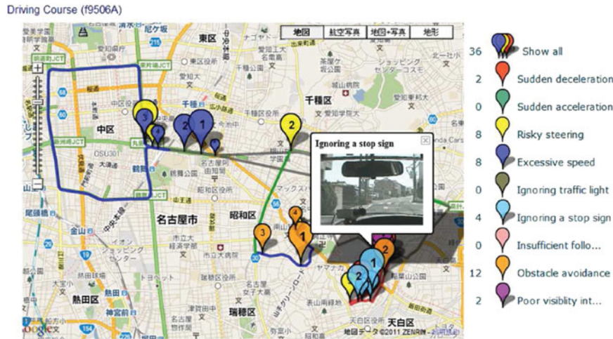
Fig. 16. Interface summarizes hazardous situations on a driving map.
