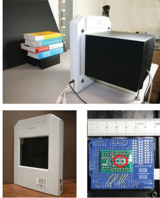
Fig. 7. Prototype device. Top: lab setup. Bottom left: the LCD screen as the aperture assembly. Bottom right: the sensor board with two sensors, indicated by the red circle.
