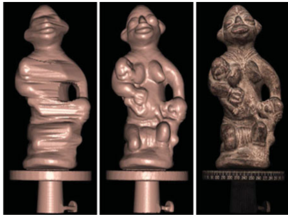
Fig. 5. VH(silhouette only) and improvement by joint-optimization of silhouette+photoconsistency (Esteban and Schmitt [31]). Left: silhouette based visual hull (low concavity). Middle: Silhouette and photoconsistency joint optimization by level-set. Right: Original input image.
