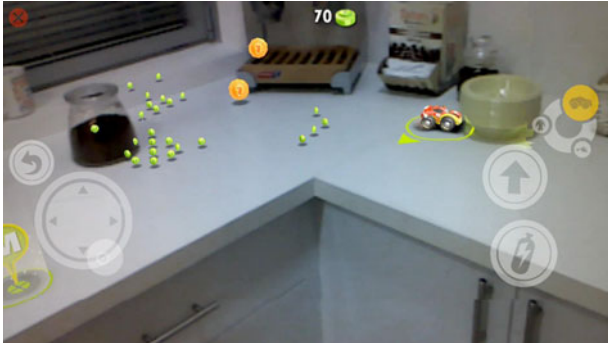
Fig. 16. Augmentation of the real physical world with virtually rendered 3D objects using a device with embedded RealSense module. Here a digitally rendered car is shown racing on a real kitchen table and colliding into a physical bowl, with realistic physical effects such as collision with real objects, correct occlusion, shadows, etc.
