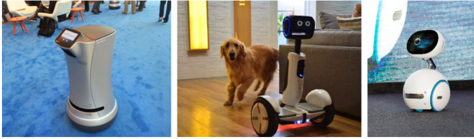
Fig. 13. Examples of autonomous robots equipped with RealSense technology. Left, a hotel butler robot from Savioke; middle, Segway personal transporter robot from Ninebot; right, a personal assistant home robot from Asus.
