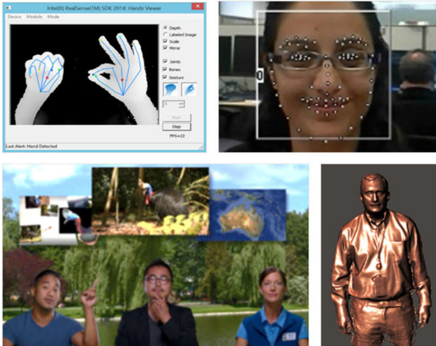
Fig. 9. Examples of 3D computer vision middleware libraries included in the RealSense software development kit. Top left: 3D hand skeleton tracking; top right: face detection and tracking; bottom left: 3D background segmentation; bottom right: 3D scanning and reconstruction.
