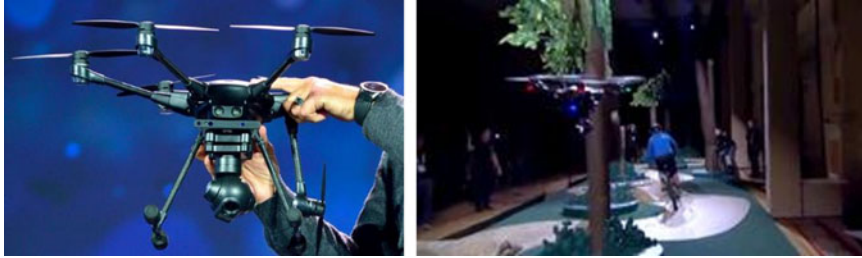
Fig. 14. The left image shows the Yuneec Typhoon H drone with integrated RealSense device as demonstrated in CES 2016. The right image shows a demonstration of real-time automatic collision avoidance as the drone follows a person biking through trees.
