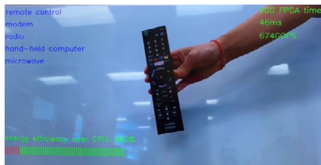
Fig. 10. Object recognition: A VGG network running on NovuMind's AI processor FPGA prototype performs real time object recognition. Upper left-hand corner lists the top-5 recognition results.
