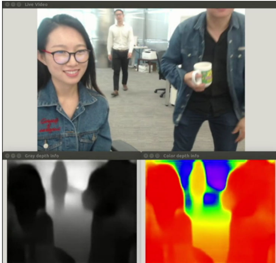
Fig. 15. Monocular depth estimation with a DNN. (Top) Input RGB image. (Bottom) Output depth map in grayscale and pseudo color.
