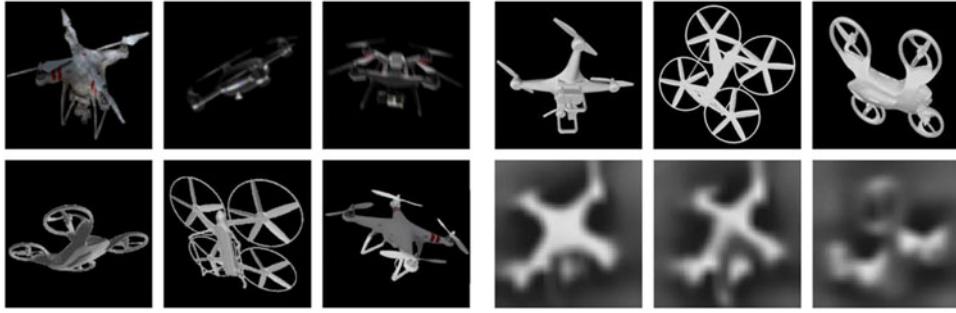
Fig. 4. Illustration of augmented visible and thermal drone models. The left three columns show the augmented visible drone models using different augmentation techniques. The right three columns show the augmented thermal drone models with the first row exploiting 3D rendering technique and the second row utilizing Generative Adversarial Networks.
