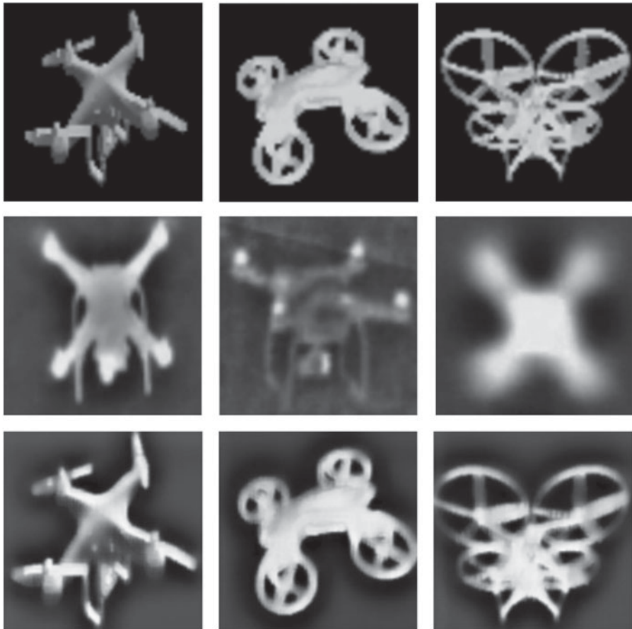
Fig. 8. Comparison of generated thermal drone images of different methods: 3D rendering (first row), Cycle-GAN (second row), proposed method (third row).
