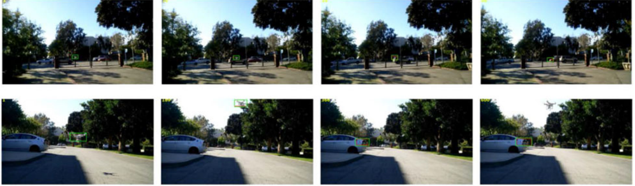
Fig. 14. Failure cases. Our algorithm fails to track the drone with strong motion blur and complex background (top row), and fails to re-identify the drone when it goes out-of-view and back (bottom row). The bounding boxes in red are integrated system results and the bounding boxes in green are tracking-only results.
