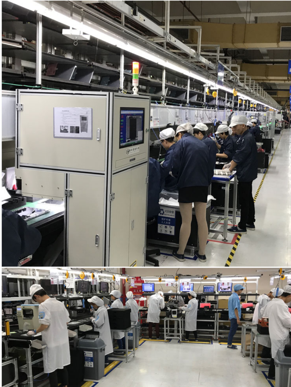
Fig. 5. A laptop system assembly facility. Top: an assembly line for higher production rate. Bottom: an assembly cell for lower yield but higher product variety.
