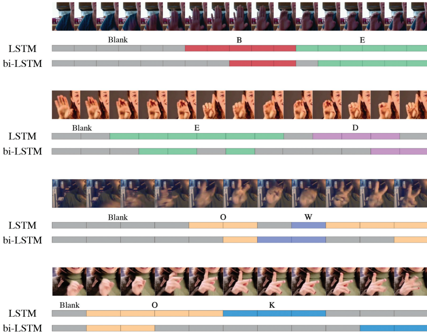
Figure 7: The comparison of the alignment result between Bidirectional LSTM and LSTM learned by CTC.
