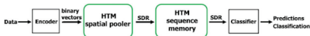
Figure 1: The basic structure of the HTM model consists of semantic encoder, spatial pooler, and temporal memory [5].
