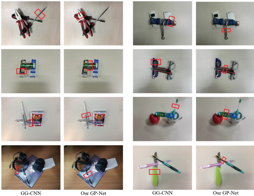
Figure 1: Comparisons of GG-CNN[25] and our GP-Net. The grasp representations of different networks in complex stacking scenarios from the VMRD dataset [46]. It can be seen that our GP-Net can focus on the top-level objects.
