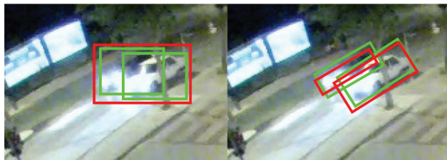
Figure 3: The normal box detector (left) fails to get the precise vehicle bounding boxes to separate two cars, but the rotated detector (right) is able to construct two tighter bounding boxes. Green box: ground truth. Red box: predicted vehicle location.
