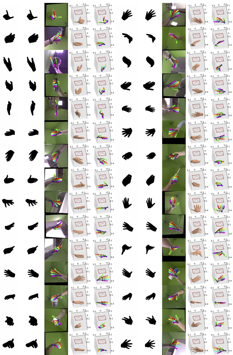
Figure 3: Each result set contains a 2D binary mask as the input, followed by the predicted mask, 2D skeleton, mesh, and 3D skeleton.
