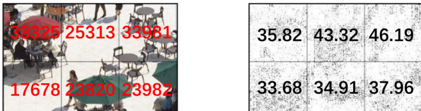
Figure 2: The bit consumption map (left) and SATD distribution of the image (right).
