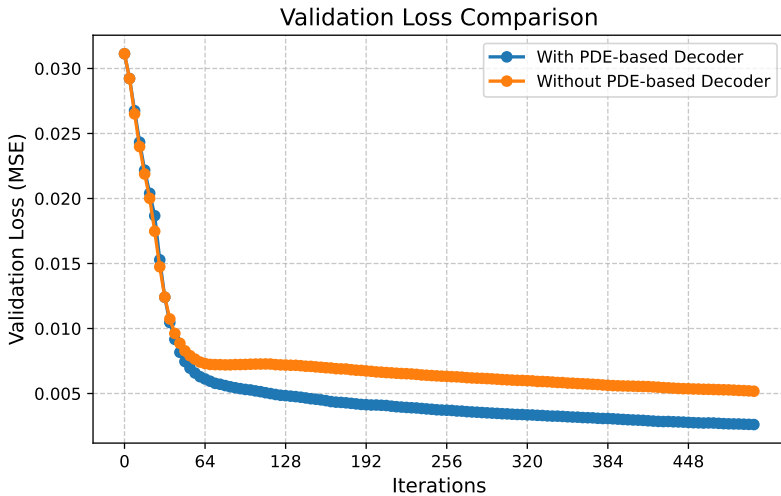
Figure 9: Comparison of validation loss of the xgboost model w/wo PDE-based decoder at the coarsest layer. The validation loss is the MSE between the predicted UDF and the ground-truth UDF.
